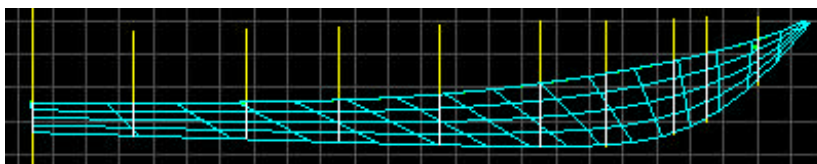
Graphical editor makes it easy to adjust keel and chine curves
